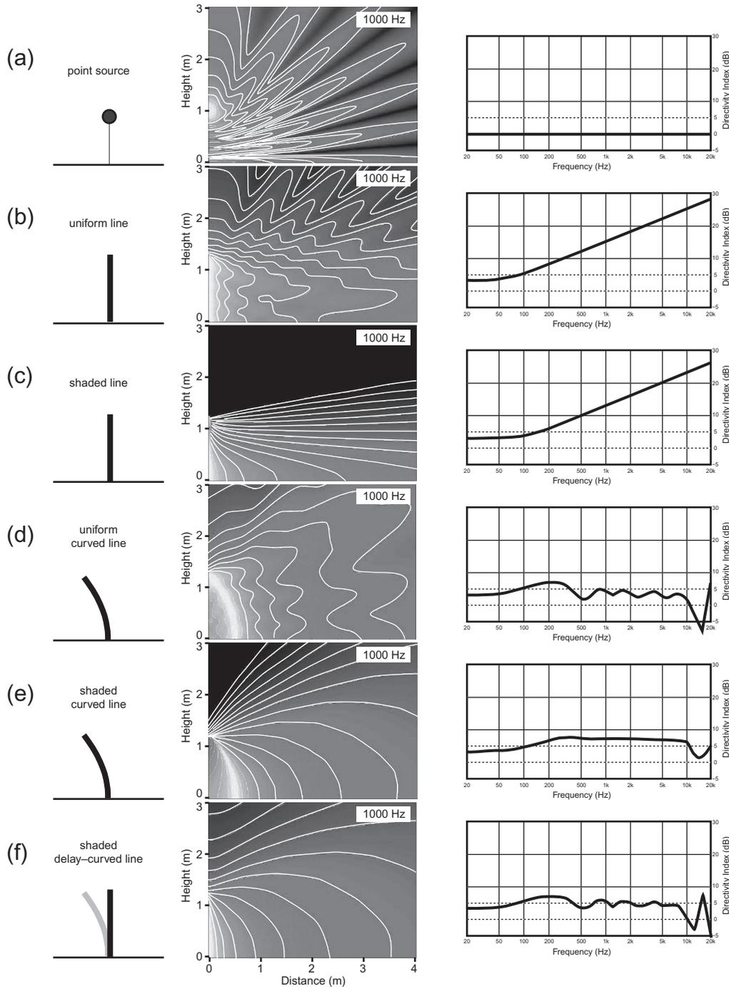
**FIGURE 18.3** Illustrations of the near-sound fields generated above a ground plane by several sound sources. The shading gets darker as sound levels drop; adjacent contour lines represent sound levels that differ by 3 dB. The original paper displays results for several frequencies; all of those shown are for 1 kHz. The words and graphics on the left explain the sources. On the right are far-field directivity indexes. Data from Keele and Button (2005).
