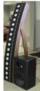
Keele's Fourth CBT Array Prototype of 2005 (Ittersbach Array). Uses all Automotive Transducers. 16 each 100mm MMX Cone Drivers and 24 each 100mm EDPL Drivers. (Electro-Dynamic Planar Loudspeaker).
