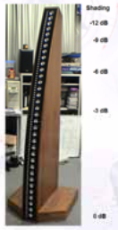
Keele's Fourth CBT Array Prototype of 2005 (Ittersbach Array). Uses all Automotive Transducers. 16 each 100mm MMX Cone Drivers and 24 each 100mm EDPL Drivers. (Electro-Dynamic Planar Loudspeaker).
