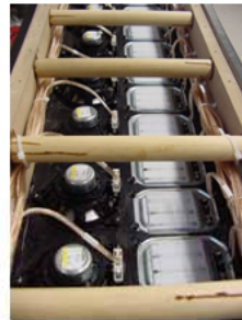
Keele's Fourth CBT Array Prototype of 2005 (Ittersbach Array). Uses all Automotive Transducers. 16 each 100mm MMX Cone Drivers and 24 each 100mm EDPL Drivers. (Electro-Dynamic Planar Loudspeaker).
