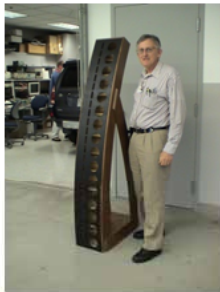
Keele's Fourth CBT Array Prototype of 2005 (Ittersbach Array). Uses all Automotive Transducers. 16 each 100mm MMX Cone Drivers and 24 each 100mm EDPL Drivers. (Electro-Dynamic Planar Loudspeaker).
