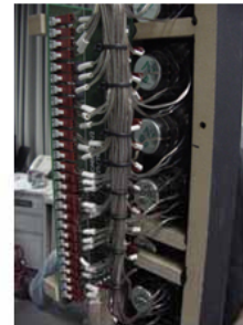
Keele's Fourth CBT Array Prototype of 2005 (Ittersbach Array). Uses all Automotive Transducers. 16 each 100mm MMX Cone Drivers and 24 each 100mm EDPL Drivers. (Electro-Dynamic Planar Loudspeaker).
