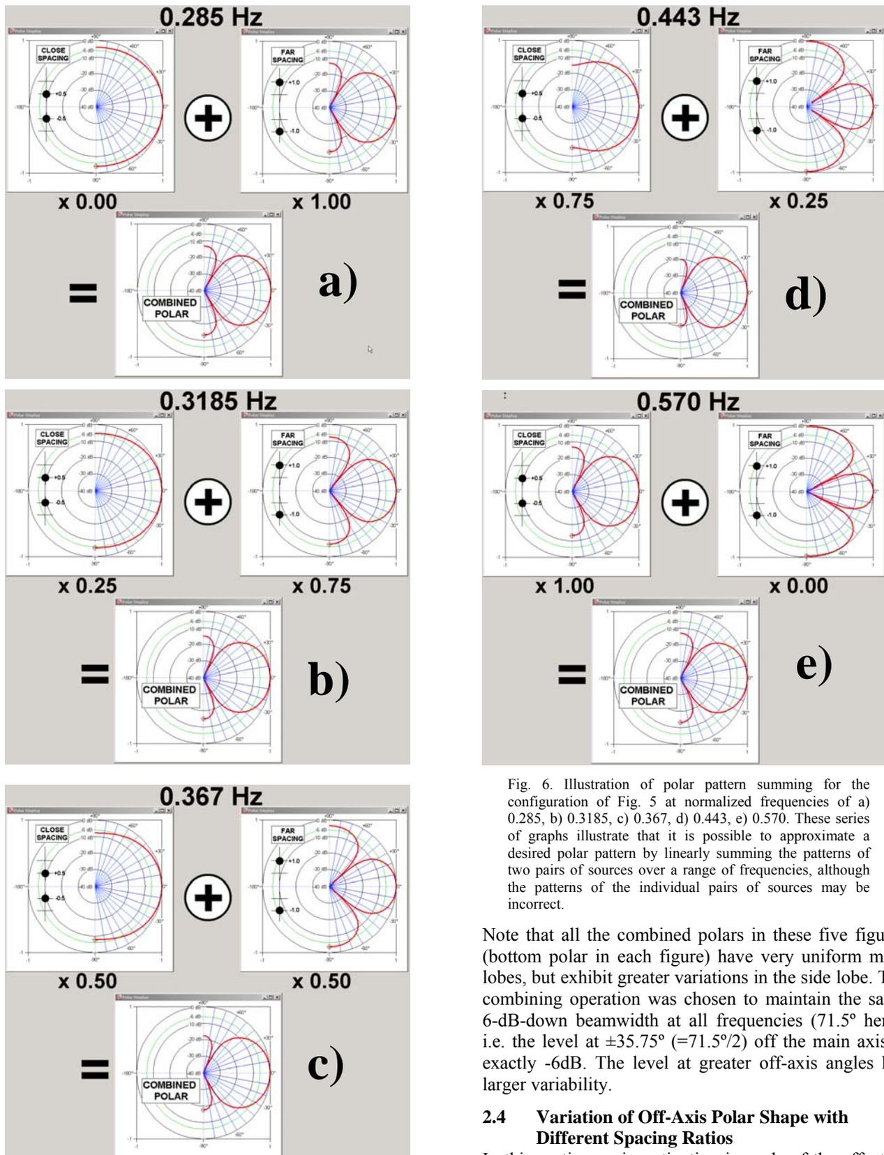
Fig. 6. Illustration of polar pattern summing for the configuration of Fig. 5 at normalized frequencies of a) 0.285, b) 0.3185, c) 0.367, d) 0.443, e) 0.570. These series of graphs illustrate that it is possible to approximate a desired polar pattern by linearly summing the patterns of two pairs of sources over a range of frequencies, although the patterns of the individual pairs of sources may be incorrect.
