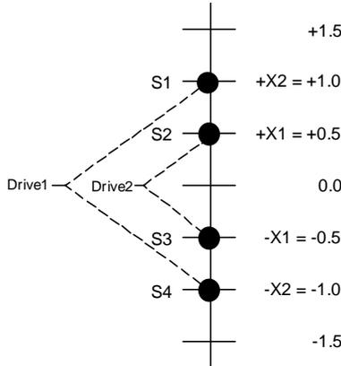
Fig. 5. Configuration of four point sources (S1 - S4) oriented vertically at normalized locations of -1.0, -0.5, +0.5, and +1.0 and driven in pairs: Drive1 to S1 and S4, and Drive2 to S2 and S3. At the lower critical normalized frequency of 0.285, the outermost sources S1 and S4 are separated by 0.57 wavelength. Correspondingly, at the higher critical frequency which is twice as high, the innermost sources S2 and S3 are also separated by 0.57 wavelength.
