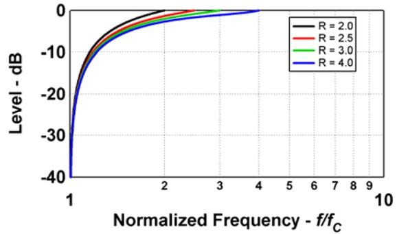
Fig. 10. High-pass crossover responses for several critical frequency ratios: (left to right) R = 2.0, 2.5, 3.0, and 4.0, calculated using Eq. 6.
