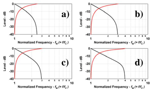
Fig. 11. Low-pass (black) and high-pass (red) crossover responses for a critical frequency ratios of a) 2, b) 2.5, c) 3.0, and d) 4.0.
