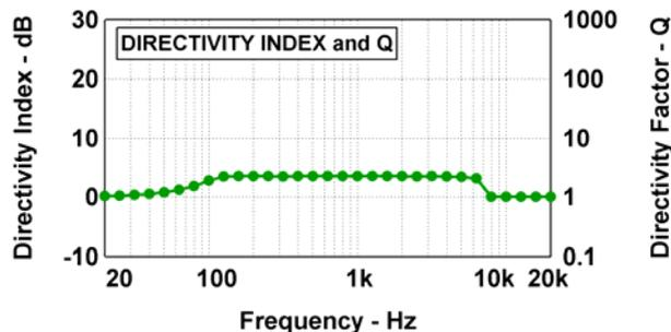
Fig. 18. Directivity versus frequency of the example five-way constant-beamwidth speaker system shown in Fig. 15. Note the extremely uniform +3.5 dB directivity index between 125 Hz and 6.3 kHz. The directivity drops above 6.3 kHz due to the omni-directional tweeter which is operating alone. The pass-band directivity can potentially be 3 dB higher depending on how the rear radiation is attenuated.
