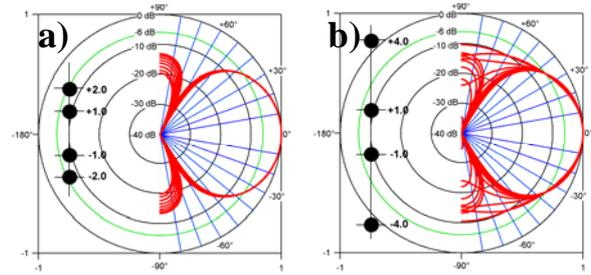
Fig. 8. Polar pattern overlays for pairs of sources separated by different spacing ratios for a critical design wavelength of  $0.57 \lambda$ : a) ratio = 2:1, and b) ratio = 4:1. To generate each polar overlay, the frequency was varied in 10 steps between the two critical frequencies so as to maintain a constant beamwidth of 71.2°. Although this critical design wavelength has a lobe at  $\pm 90^\circ$ . The main lobe is still much more uniform for the smaller spacing ratio.
