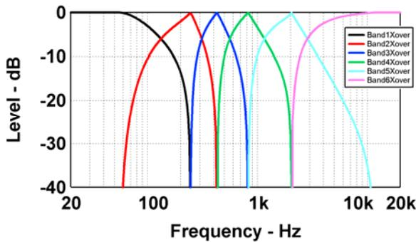
Fig. 1. Crossover frequency responses for a six-way speaker system following the design technique of part 1. Each band's crossover only drives a single pair of speakers. At any specific frequency, only a single pair of drivers or at most two pairs of drivers are operating. At the pointed peak of each crossover band, called a critical frequency, only one pair of drivers are operating. This crossover has critical frequencies of [56, 247, 430, 824, and 2060] Hz.
