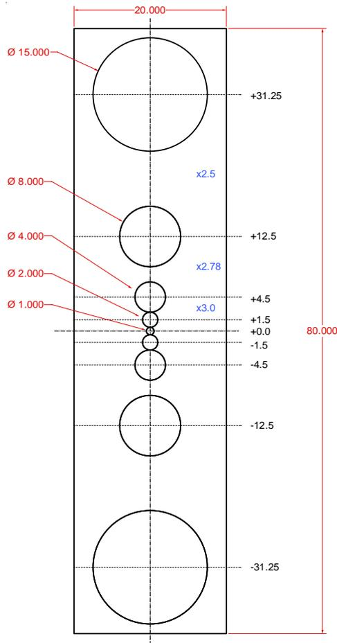
Fig. 15. Driver locations and front panel layout for the example five-way constant-beamwidth loudspeaker system. The system uses two 15” sub woofers, two 8” woofers, two 4” lower midranges, two 2” upper midranges, and a single 1” dome tweeter. The driver spacing ratios are indicated with “x” prefixes. All dimensions in inches.
