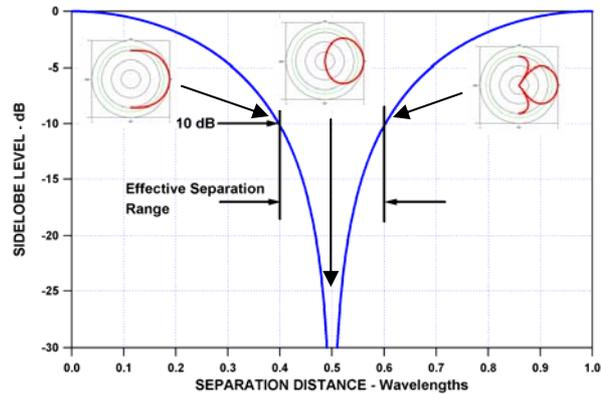
Fig. 4. Side lobe level (at  $\pm 90^\circ$ ) vs. separation distance for two point sources. For design purposes, effective source separations between 0.4 to 0.6 wavelength yield side lobes that are 10 dB down or lower. A separation distance of one-half wavelength ( $D = 0.5 \lambda$ ) results in no side lobes. Example mini polar patterns are shown at the extremes and center of the suggested design range.
