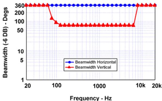
Fig. 17. Beamwidth (-6 dB) versus frequency of the example five-way constant-beamwidth speaker system shown in Fig. 15. Note the extreme uniformity of beamwidth which is about 75° between 125 Hz and 6.3 kHz. At 7.4 kHz and above, the tweeter (assumed to be a point source) is radiating by itself and provides an omni-directional 180° response. This can be corrected by using a tweeter with an inherent controlled high-frequency coverage.
