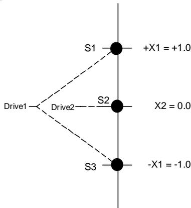
Fig. 12. Configuration of three point sources ( $S_1 - S_3$ ) oriented vertically at normalized locations of -1.0, 0.0, and +1.0. The outside pair is driven by Drive1 (low pass) and the single inside source is driven by Drive2 (high pass). Note that the source strength of the center point source is twice that of the adjacent sources thus making their farfield pressure contributions equal.
